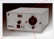
Linear readout accurately displays output from 0-100%. Switch selectable scale can be set to read voltage or Intensity.
