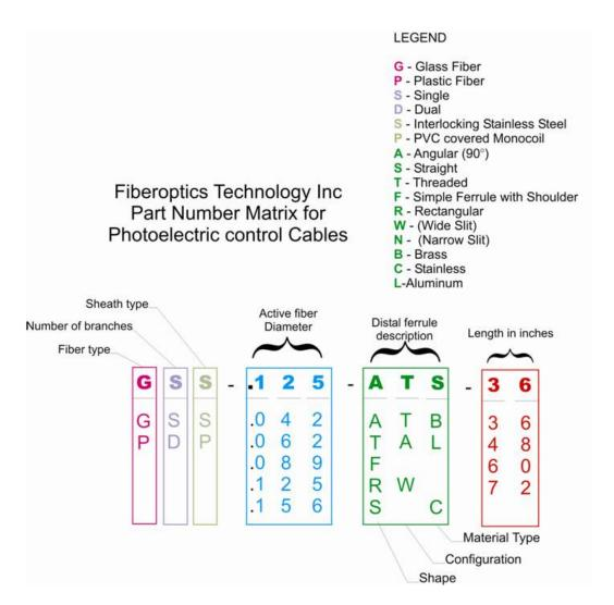
To use the matrix, choose the appropriate letter or number in order. The distal ferrule description (Green) can be any number of descriptive letters, but the order is important.... in the example above..."AT" signifies an Angular (90 degree) end tip with Threads. If it is described as "TA", the distal ferrule would have a Threaded section first, followed by the Angular portion.
