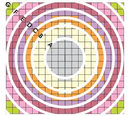
Extension harness tails are color coded to identify length. Use the grid above and the harness chart (Top left) to identify length by color.
