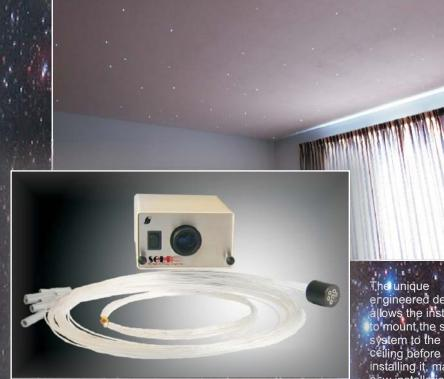
The StarScape system is comprised of three components: the light source, a SOL-R 3575 reconfigurable quartz halogen power supply which accepts 35,50, or 75W 12 volt MR16 lamps, the preassembled and polished extension harness and various star bundles. 16 standard stocked parts can create star fields ranging In size from 100 to 1200 sq feet in area, with densities ranging from 5 to 5 stars per sq foot.
